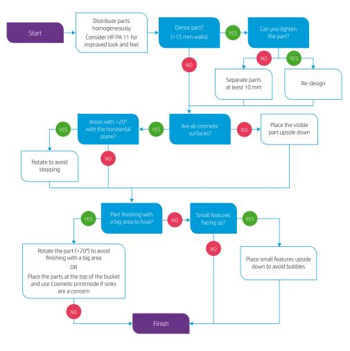
Figure 6. Flowchart for an appropriate process-parameter selection based on the geometry and functionality of a part in order to maximize its look and feel
