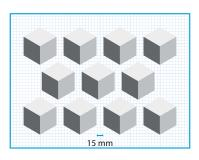
Figure 3. Recommended distance between dense parts
