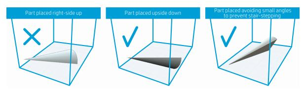
Figure 2. Orientation strategies for parts displaying curved areas to minimize the appearance of excessive layer discretization
